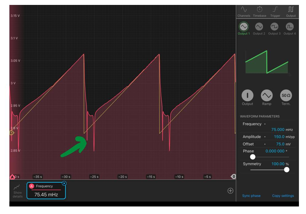
The dips pointed to in green arrows are a result of the temperature going up (temperature graph would be inverted from the yellow) from the signal drop, which means the scan passes through the absorption dip again. These signals are not well-resolved since the response time causes the absorption dips to start overlapping. They were not included in the analysis.
